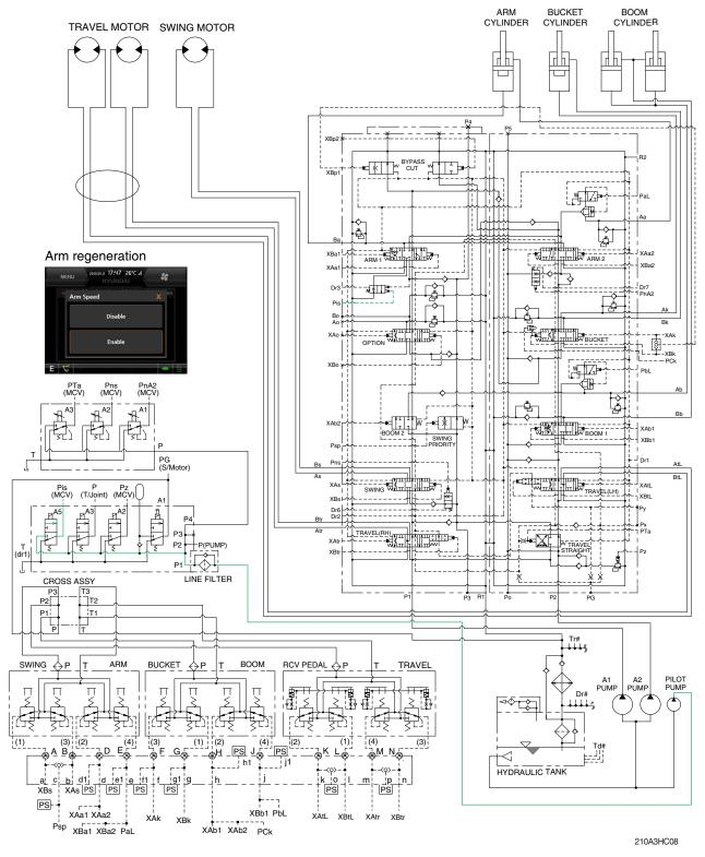
When the arm regeneration is selected to disable on the cluster, the arm regeneration solenoid valve is activated. The pilot oil from pilot pump flow into **Pis** port in main control valve through solenoid valve and the arm regeneration spool is shifted to left.
