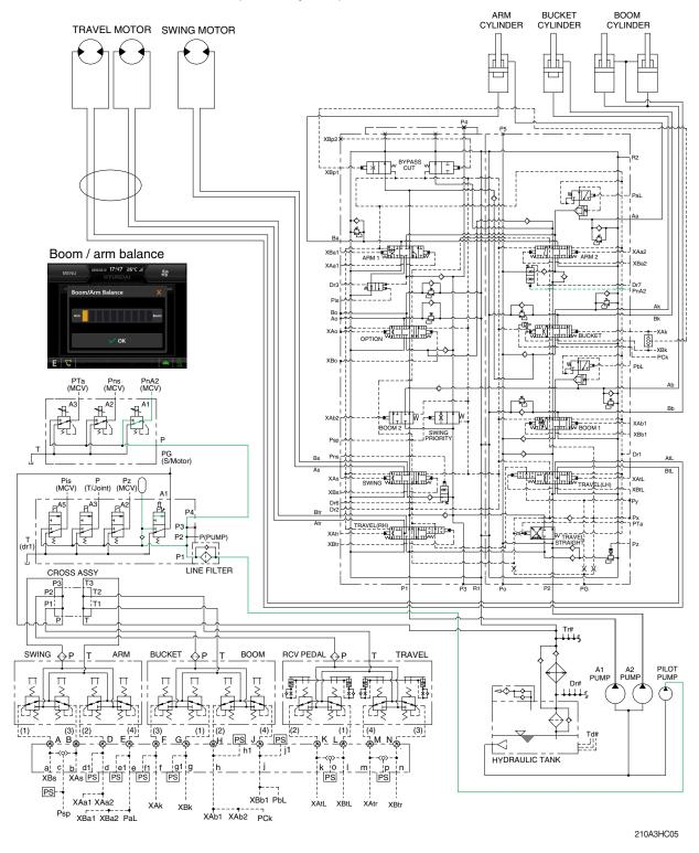
When carrying out the combined operation of boom up and arm in, the boom up operating speed is lowered then normal operation.
